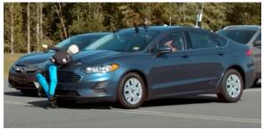
Figure 2: Child Pedestrian Target during Impact [2]
